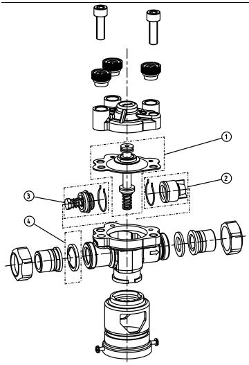
Fig. F-1: Spare parts for Euro system separator GENO-DK 2-Mini
