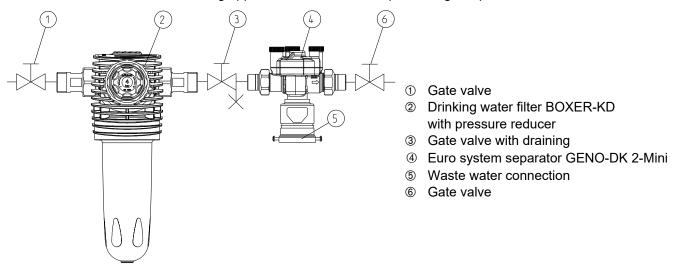
Fig. D-1: Installation example: filter combination of fine filter BOXER-KD with Euro system separator GENO DK 2
