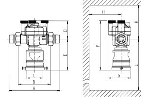
Fig. C-2: Dimensional drawing of Euro system separator GENO-DK 2-Mini
